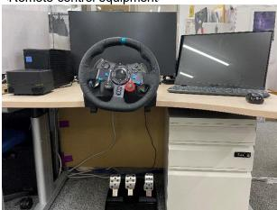
The driver can safely operate the vehicle using the steering wheel and pedals while viewing images of the vehicle's surroundings projected on the screen and Al-based object detection information.
