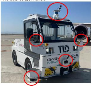
The system is equipped with a device that uses LIDAR sensors outside the vehicle to safely stop the vehicle even during remote operation, based on information about the driving area captured in the system beforehand.
