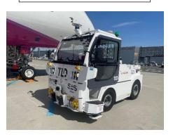
The "X-Area Remote" control system developed by Panasonic HD will be used to control travel within the ramp area of Terminal 2 using public mobile lines (4G/5G) from terminals installed in Peach's Aeroplaza office.
