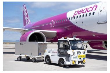
This demonstration test aims to verify the practicality of vehicle operation using autonomous driving technology within the ramp area—marking the first such initiative at Kansai Airport. The trial uses the "EZTow" vehicle manufactured by Tracteasy, provided by Nagase Techno Level 3 autonomous driving test has been conducted from December 2024 through April 20, 2025, and a Level 4 autonomous driving test is currently underway<sup>\*2</sup>.
